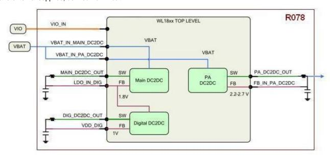
Figure 3-3 Internal DC2DC's
