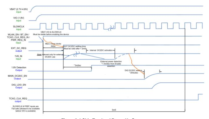
Figure 3-4 Chip Top-level Power Up Sequence
