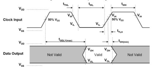
Figure 4-4 SDIO HS output timing
