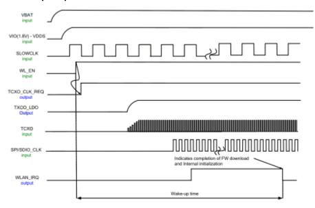
Figure 3-5 WLAN Power Up Sequence
