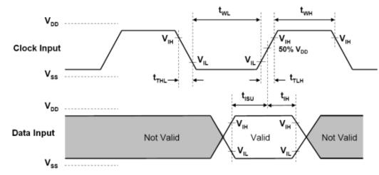
Figure 4-3 SDIO HS input timing
