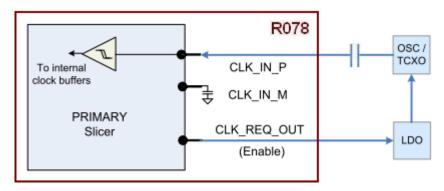
Figure 3-2 Fast Clock Block Diagram
