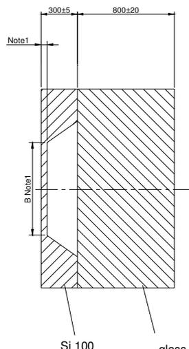
Note1: geometry of diaphragm depend on specification
