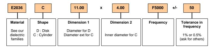
Example for dielectric resonator with spacer in dimension: E2036/AL C 11.00x4.00x5.35
