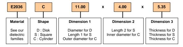
Example for dielectric resonator in frequency: E2036 C 11.00x4.00 F5000+/-50
