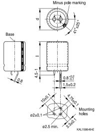
Snap-in capacitors are also available with 3 terminals (length (4.5 –1) mm). PET insulation is marked with label "PET" on the sleeve. Safety vent on the case wall.
