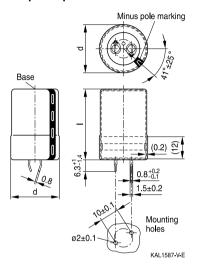
Snap-in terminals, length (6.3 + 1/-1.4) mm. Also available in a shorter version with a length of (4.5 - 1.4) mm. PET insulation cap is positioned under the insulation sleeve. Safety vent on the case wall.
