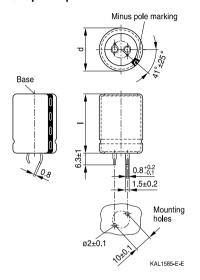
Snap-in terminals, length ( $6.3\pm1$ ) mm. Also available in a shorter version with a length of (4.5-1) mm. PET insulation is marked with label "PET" on the sleeve. Safety vent on the base or on the case wall.
