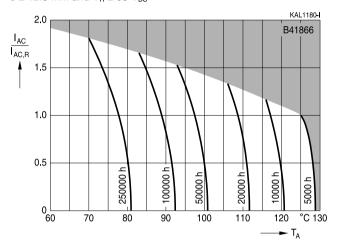
Useful life $^{1)}$  depending on ambient temperature  $T_A$  under ripple current operating conditions  $V_R = 75 \ V_{DC}$
