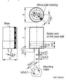
Snap-in terminals, length (6.3 + 1/-1.4) mm. Also available in a shorter version with a length of (4.5 - 1.4) mm. PET insulation cap is positioned under the insulation sleeve.
