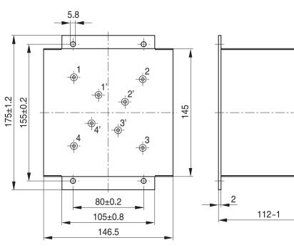
Tolerances to ISO 2768-C unless otherwise noted. Dimensions in mm
