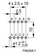
Recommended hole arrangement (view in mounting direction)
