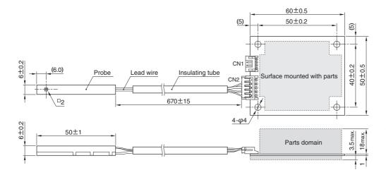
CN1 S4B-PH-KLC-H(LF)(SN) JST Connector (I/O pins)
