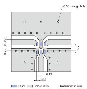
Line width should be designed to match  $50\Omega$  characteristic impedance, depending on PCB material and thickness.
