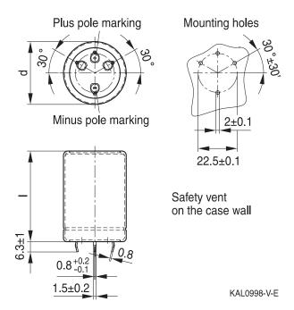
Standard snap-in terminals: length (6.3  $\pm$ 1) mm. Also available with length of (4.5 -1) mm.
