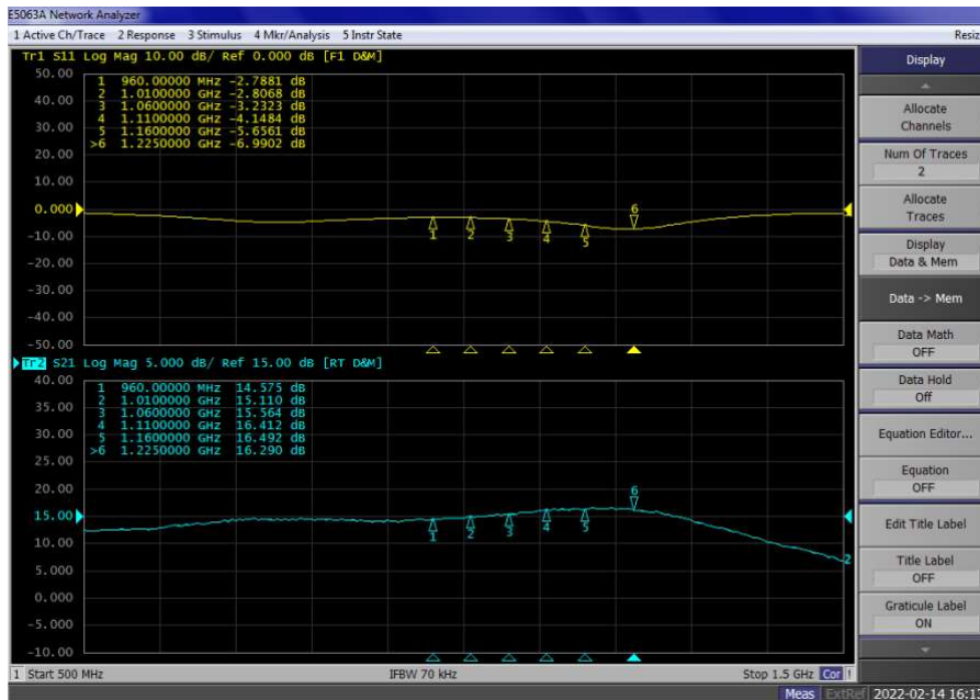
Figure 2. Network analyzer output S11/S21
